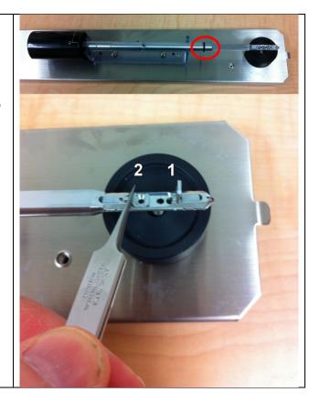
4. Place the specimen rod into the airlock by aligning the pin on the specimen rod with the slot on the airlock (black arrow) and inserting until a click is heard.
