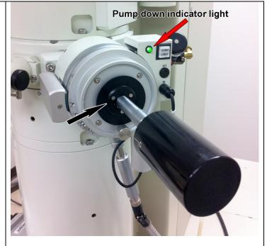
5. Turn on the filament by pressing the FIL button (17, on the Right Control Panel)
