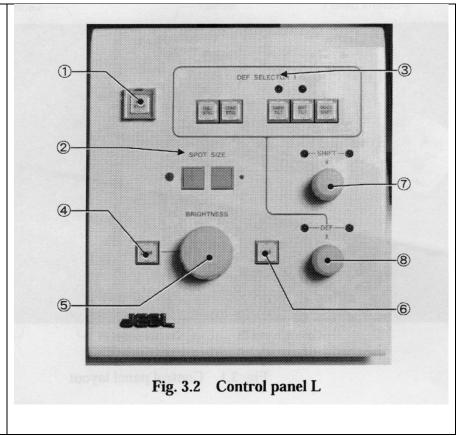
The **Spot size** can be changed to suit the method of imaging and brightness levels by pressing the buttons (#2). Typical operation is at spot size 2.
